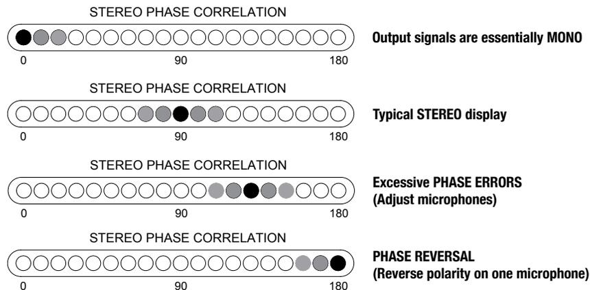
And, whether using M-S, X-Y or other stereo mic techniques, our Stereo Phase Correlation Display can assist in positioning the microphones for a rich stereo image. The Stereo Phase Correlation circuit "listens" to the two preamp outputs in the frequency range where human hearing is most sensitive to audio phase information. It analyzes the phase information and displays the following conditions:
